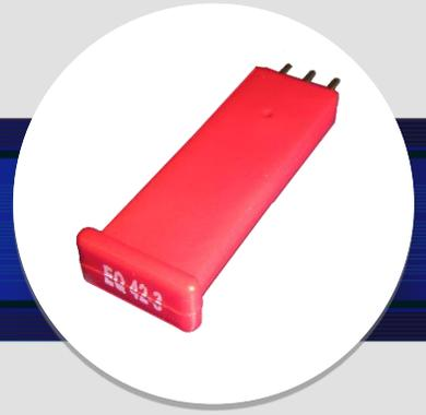
The Reverse JXP style Equalizer is normally installed at the input RF flow of the upstream optical transmitter located inside the optical node. The optical node is located in the outside cable plant in most CATV system and connected to the Headend via a fiber optic cable. This equalizer allows the signals to be pre-equalized before reaching the headend.
