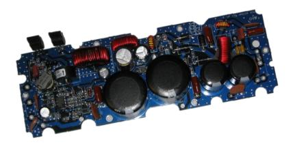
The power supply is a fixed frequency-switching regulator that allows for a superior power factor to the 37-90 volt input line. The 29PS000 BBI power supply is installed in the back of the BBI or OEM RF amplifier module. The module must be removed from the field for repair.
