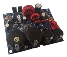
The regulator is a fixed frequency-switching regulator that allows for a superior power factor to the 40-90 volt input line. The power supply requires a soldering station for removal of the old defective unit and placement of the new power supply. The 214PS000 BBI power supply is installed in the back of the BBI 4PAC amplifier module, and the amplifier module must be removed from the field for repair.
