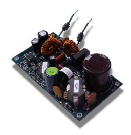
The power supply is a fixed frequency-switching regulator that allows for a superior power factor to the 37-90 volt input line. The 25PS000 BBI power supply is installed in the center of the BBI 2PAC-G, S, or S2 amplifier module, and the amplifier module must be removed from the field for repair.
