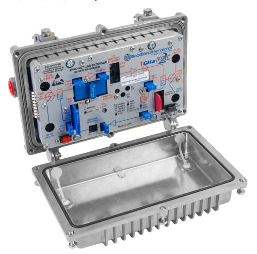
The 2PAC-MOT Super High Gain (SGaN) enhanced system amplifier module from Broadband International® is designed to drop into your existing JLX and BLE line extender housing. The forward bandwidth is up to 1 GHz and may be optimized for any bandwidth from 550 to 1 GHz. This is accomplished by alignment of the interstage response network and by the type of cable equalizers utilized. Performance may be optimized by the choice of GaN hybrids to achieve different operating gains.
