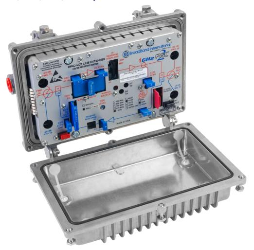
The 2PAC-MOT (RG) enhanced system amplifier module from Broadband International® is designed to drop into your existing JLX and BLE line extender housing. The forward bandwidth is up to 1 GHz and may be optimized for any bandwidth from 550 to 1 GHz. This is accomplished by alignment of the interstage response network and by the type of cable equalizers utilized. Performance may be optimized by the choice of GaN hybrids to achieve different operating gains.
