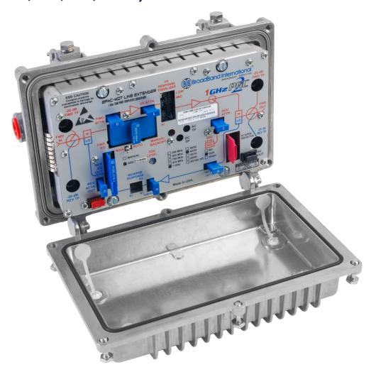
The 2PAC-MOT High Gain (GaN) enhanced system amplifier module from Broadband International<sup>®</sup> is designed to drop into your existing JLX and BLE line extender housing. The forward bandwidth is up to 1 GHz and may be optimized for any bandwidth from 550 to 1 GHz. This is accomplished by alignment of the interstage response network and by the type of cable equalizers utilized. Performance may be optimized by the choice of GaN hybrids to achieve different operating gains.
