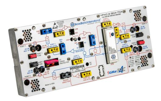
The 4PAC-M TNA 2-output enhanced system amplifier module from Broadband International® is designed to drop into any existing ARRIS®/Philips®/Magnavox® TNA system amplifier housing. The forward bandwidth is up to 1 GHz and may be optimized for any bandwidth from 550 to 1 GHz. This is accomplished by alignment of the interstage response network and by the type of cable equalizers utilized. Performance may be optimized by the choice of GaAs hybrids to achieve different operating gains.
