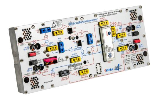
The 4PAC-M GNA 2-output enhanced system amplifier module from Broadband International® is designed to drop into any existing ARRIS®/Philips®/Magnavox® GNA system amplifier housing. The forward bandwidth is up to 1 GHz and may be optimized for any bandwidth from 550 to 1 GHz. This is accomplished by alignment of the interstage response network and by the type of cable equalizers utilized. Performance may be optimized by the choice of GaAs hybrids to achieve different operating gains.
