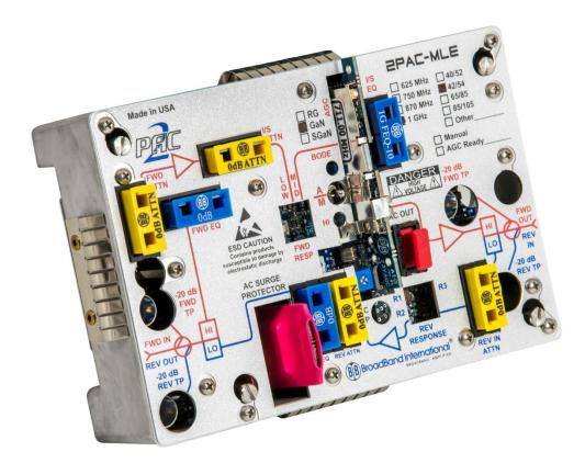
The Super High Gain 2PAC-MLE enhanced system amplifier module from Broadband International® is designed to drop into any existing Magnavox® line extender housing. The forward bandwidth is up to 1 GHz and may be optimized for any bandwidth from 550 to 1 GHz. This is accomplished by alignment of the interstage response network and by the type of cable equalizers utilized. Performance may be optimized by the choice of GaN hybrids to achieve different operating gains.
