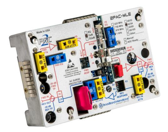
The High Gain (GaN) 2PAC-MLE enhanced system amplifier module from Broadband International® is designed to drop into your existing Magnavox® line extender housing. The forward bandwidth is up to 1 GHz and may be optimized for any bandwidth from 550 to 1 GHz. This is accomplished by alignment of the interstage response network and by the type of cable equalizers utilized. Performance may be optimized by the choice of GaN hybrids to achieve different operating gains.
