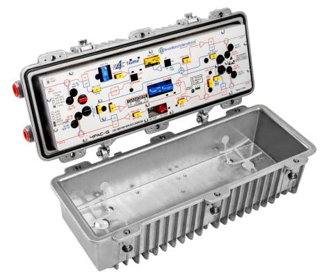
The 4PAC-G UBT enhanced system amplifier module from Broadband International® is designed to drop into any existing SA II, III or GainMaker® system amplifier housing. The forward bandwidth is up to 1 GHz and may be optimized for any bandwidth from 550 to 1 GHz. This is accomplished by alignment of the interstage response network and by the type of cable equalizers utilized. Performance may be optimized by the choice of hybrids to achieve different operating gains.
