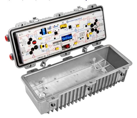
The 4PAC-G LGD enhanced system amplifier module from Broadband International® is designed to drop into any existing SA II, III or GainMaker® system amplifier housing. The forward bandwidth is up to 1 GHz and may be optimized for any bandwidth from 550 to 1 GHz. This is accomplished by alignment of the interstage response network and by the type of cable equalizers utilized. Performance may be optimized by the choice of hybrids to achieve different operating gains.
