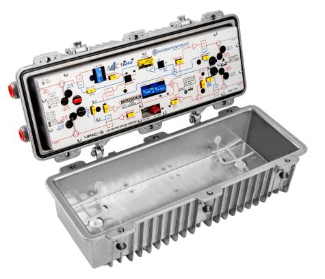
The 4PAC-G LGD enhanced system amplifier module from Broadband International<sup>®</sup> is designed to drop into any existing SA II, III or GainMaker<sup>®</sup> system amplifier housing. The forward bandwidth is up to 1 GHz and may be optimized for any bandwidth from 550 to 1 GHz. This is accomplished by alignment of the interstage response network and by the type of cable equalizers utilized. Performance may be optimized by the choice of hybrids to achieve different operating gains.
