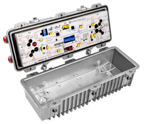
The 4PAC-G HGD enhanced system amplifier module from Broadband International<sup>®</sup> is designed to drop into any existing SA II, III or GainMaker<sup>®</sup> system amplifier housing. The forward bandwidth is up to 1 GHz and may be optimized for any bandwidth from 550 to 1 GHz. This is accomplished by alignment of the interstage response network and by the type of cable equalizers utilized. Performance may be optimized by the choice of hybrids to achieve different operating gains.
