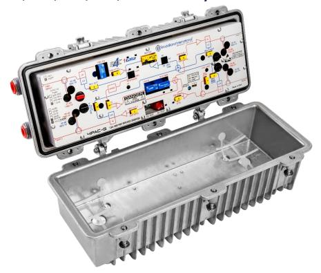
The 4PAC-G HGBT enhanced system amplifier module from Broadband International® is designed to drop into any existing SA II, III or GainMaker® system amplifier housing. The forward bandwidth is up to 1 GHz and may be optimized for any bandwidth from 550 to 1 GHz. This is accomplished by alignment of the interstage response network and by the type of cable equalizers utilized. Performance may be optimized by the choice of hybrids to achieve different operating gains.
