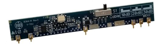
Broadband International's TDU/V can be installed in any Commscope® Motorola®, or Arris® amplifier product that has an existing location for a Vertical Automatic Drive Unit (ADU/V).
